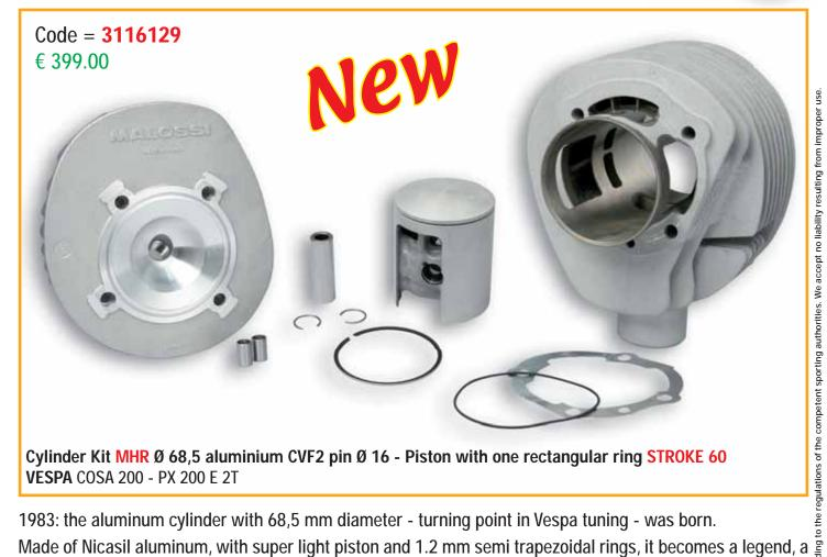
Cylinder Kit MHR Ø 68,5 aluminium CVF2 pin Ø 16 - Piston with one rectangular ring STROKE 60 **VESPA** COSA 200 - PX 200 E 2T
